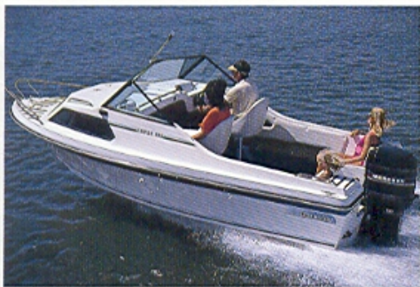
CAPRI 533 LOA 5.33m 17'7" Max Beam 2.28m 7'6" Rec. Max H.P. 150HP
