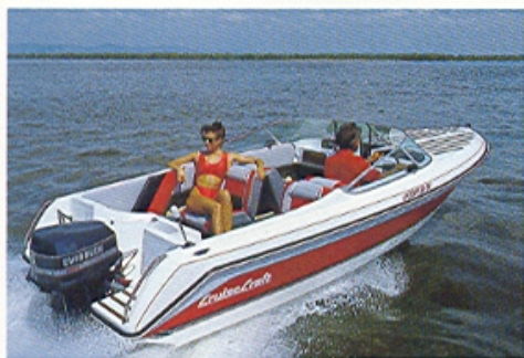
LAZER 520 Sports Runabout LOA 5.33m 17'7" Max Beam 2.27m 7'5" Rec. Max H.P. 150HP
